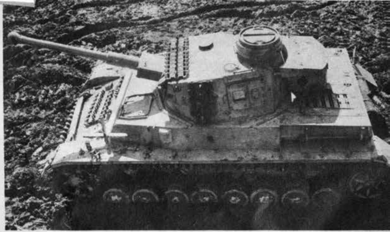
Without spaced armor Mark IV turret is angular and sprawling. Its top slopes down gradually toward rectangular mantlet. Tall cupola looks like spare tire. Behind hangs the stowage bin.
